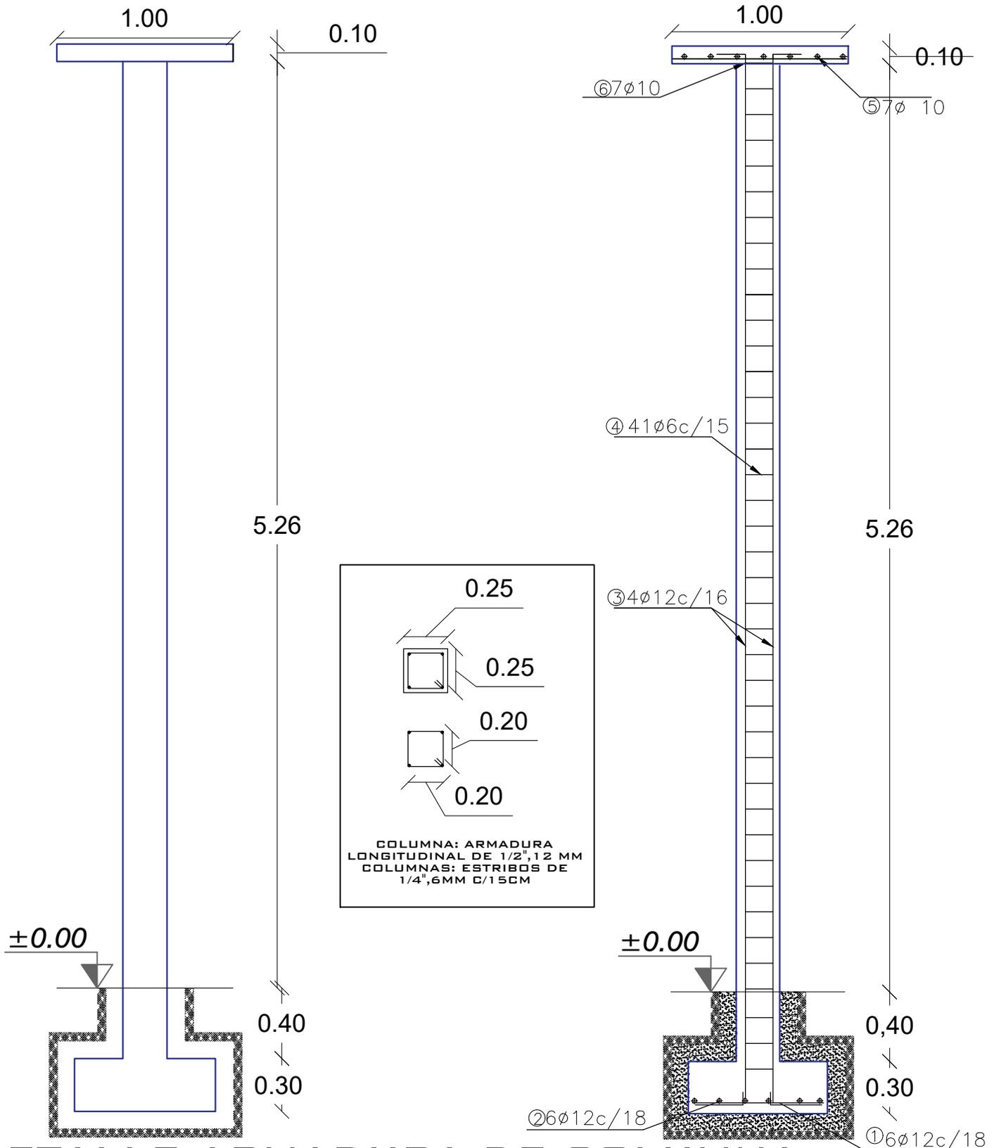
**DETALLE ARMADURA DE COLUMNA** ESC: 1:30
