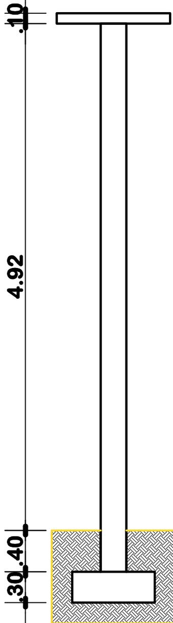
COLUMNAS: ESTRIBOS DE 1/4" - 6mm c/ 15cm
