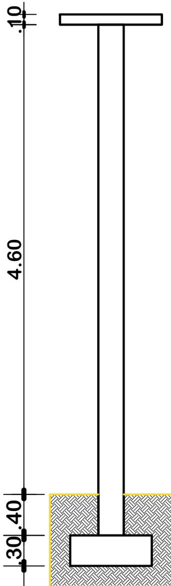
COLUMNAS: ESTRIBOS DE 1/4" - 6mm c/ 15cm
