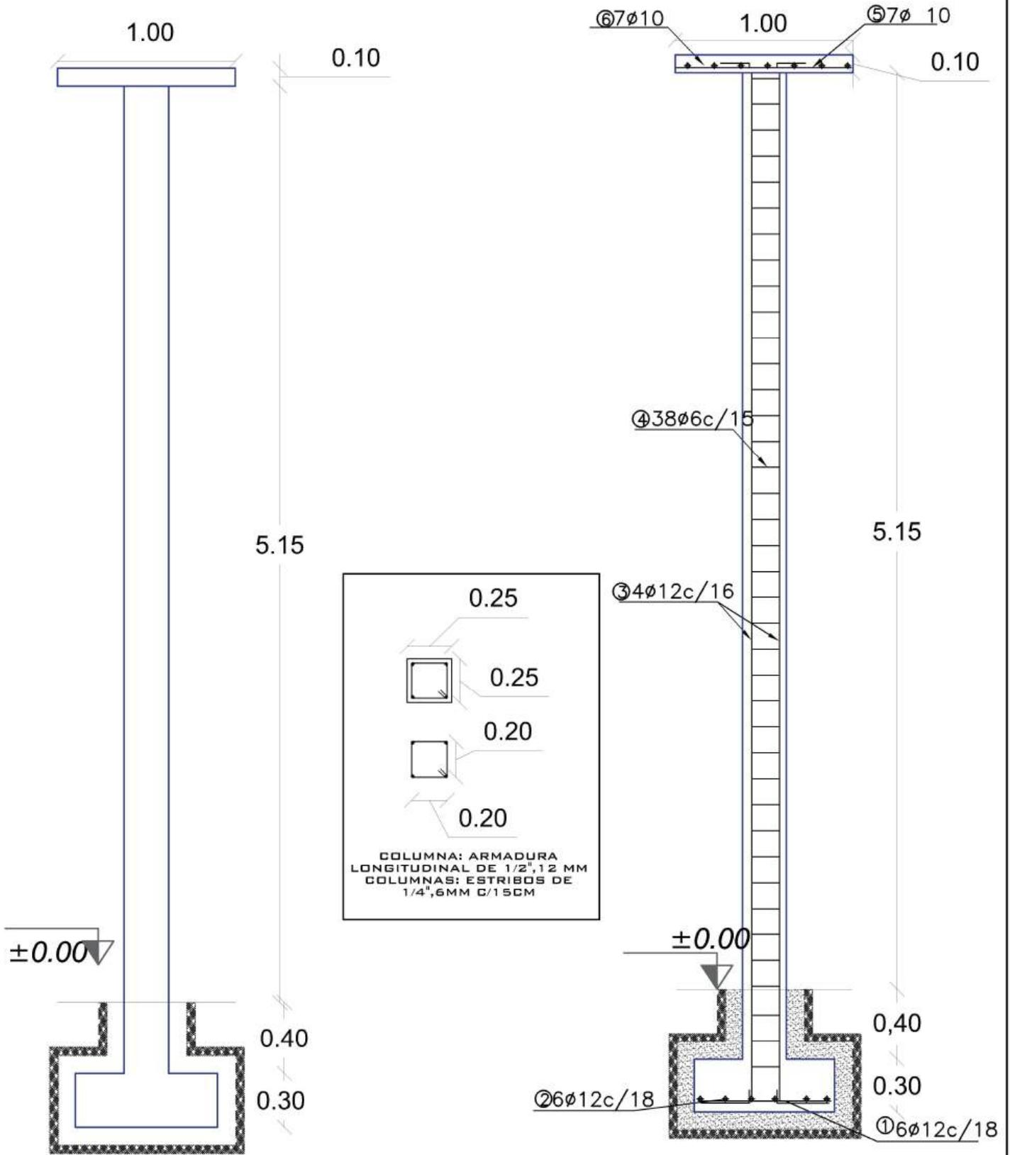
**DETALLE ARMADURA DE COLUMNA** ESC: 1:30
