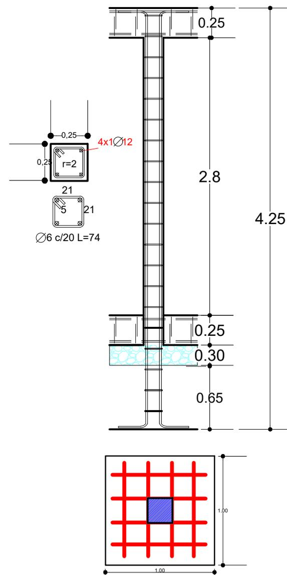
DETALLE DE COLUMNA DE TANQUE ELEVADO
