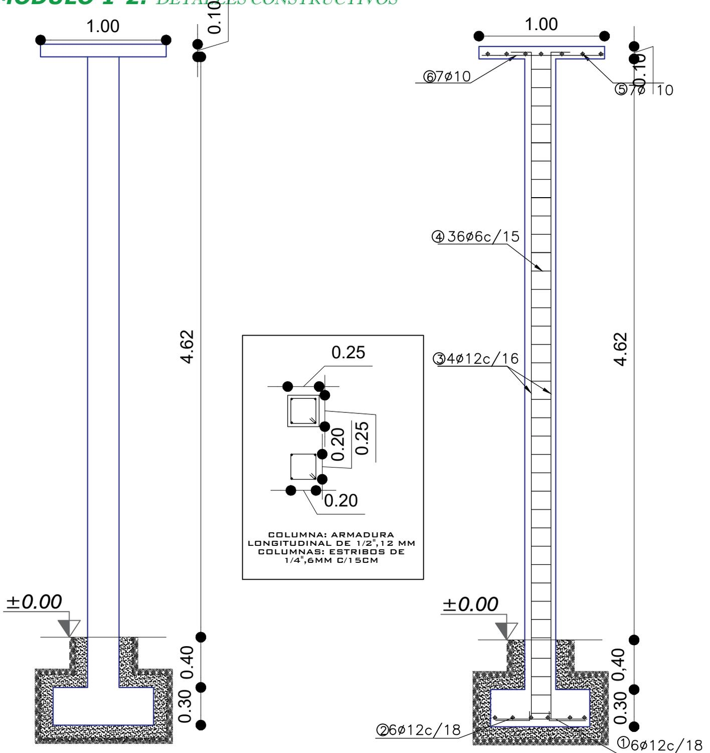
**DETALLE DE ARMADURA DE COLUMNA**
