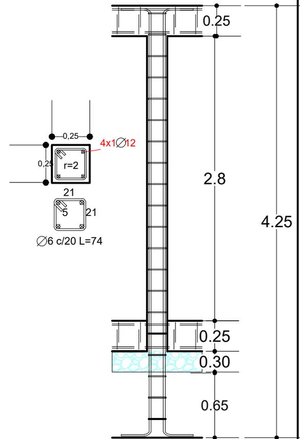
DETALLE DE COLUMNA DE TANQUE ELEVADO
