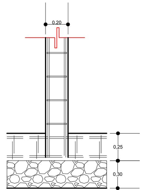
**DETALLE DE COLUMNAS QUE NACE EN VIGA**
