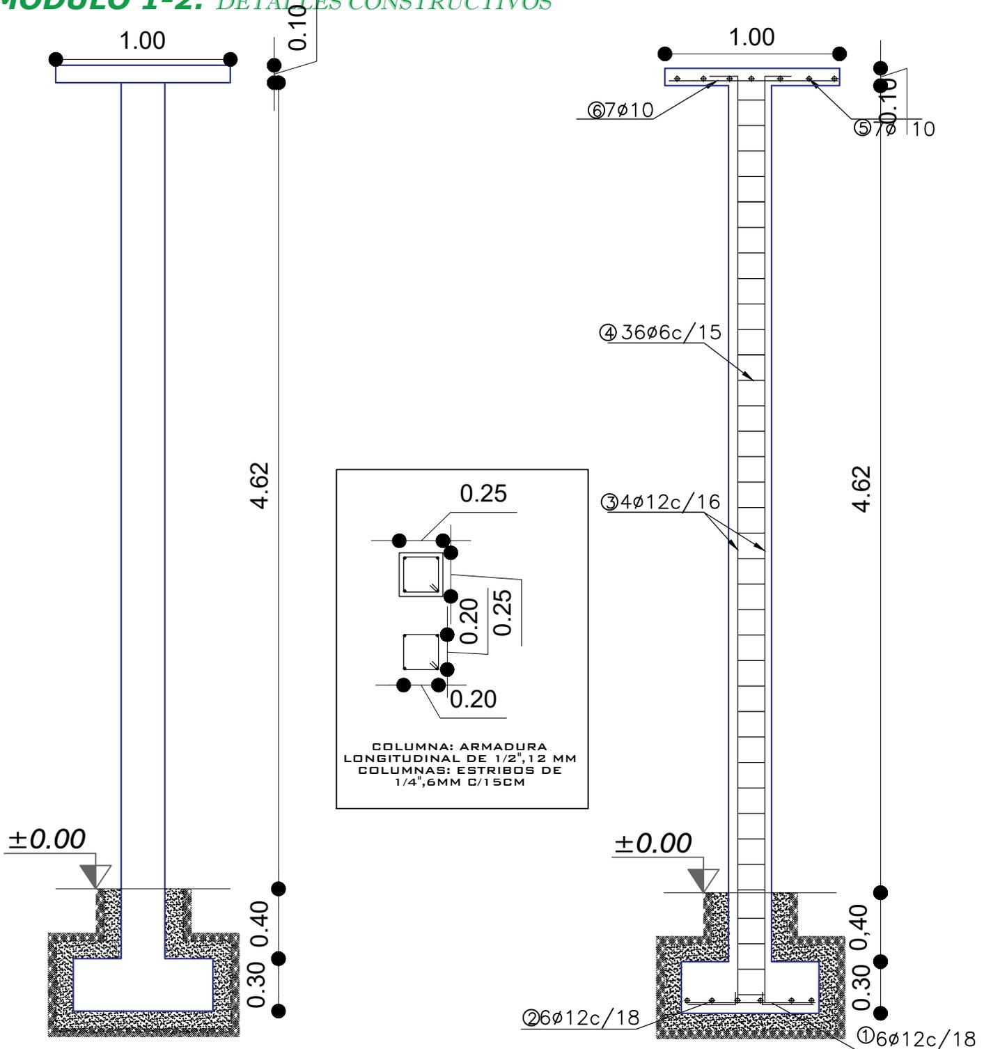
**DETALLE DE ARMADURA DE COLUMNA**
